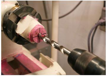
4. Using a small scraper or skew, enlarge the hole until the ring core fits snugly into the hole. Stop and check the size often to avoid making the hole too big.
