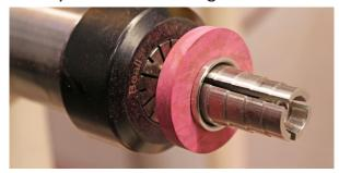
**9.** Turn the blank flush with the metal, or your desired profile.
