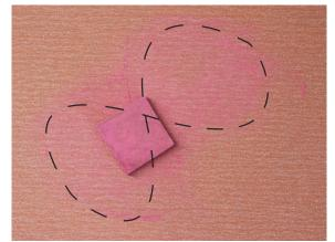
Apply 1 ½" double-sided tape to the flat surface of the ring blank and attach it to centre of the end of the trued face of the waste block.
