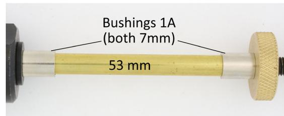
1. Assemble the blank and bushings on the mandrel.
