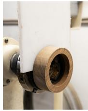
enlarging the hole. Take care not to touch the jaws of the chuck with your cutting tool.
