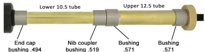
1. Assemble the blanks on the mandrel referring to the diagram above.
