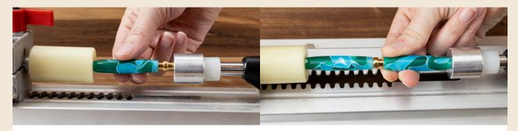
Make sure the barrels are straight when pressing them into the centerband. The passage through the centerband is narrow, so even a slight angle can cause the mechanism to catch when passing it through. Do not put excess pressure on the button or try to force the mechanism through, as this can damage the mechanism. Realign the barrels so they are straight and reinsert the mechanism.
