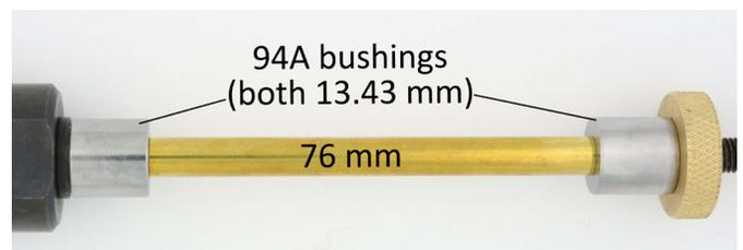
1. Put the blank on the mandrel using the 94A bushing set and by following
