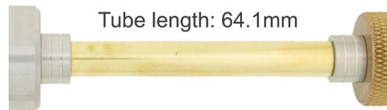
1. The nib and the clip assembly have the same diameter. Therefore both bushings are identical and can be used in either position.
