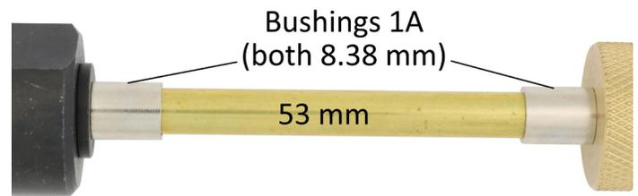
1. Assemble the blank and bushings on the mandrel.
