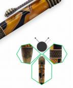
• Finish the barrel with your choice of polish. Allow sufficient time for the polish to cure.
