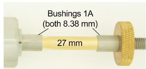
1. Assemble the blank and bushings on the mandrel.
