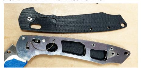
Set left liner over pivot pin and align stop pins with holes.
