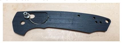
Start with the right handle (the one with pocket clip screw holes) and place the female end of the lock into the slot.
