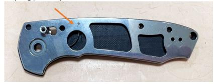
Place the liner over the top of the lock and spring while fitting the pointed tip of the spring into the small spring hole in the liner.
