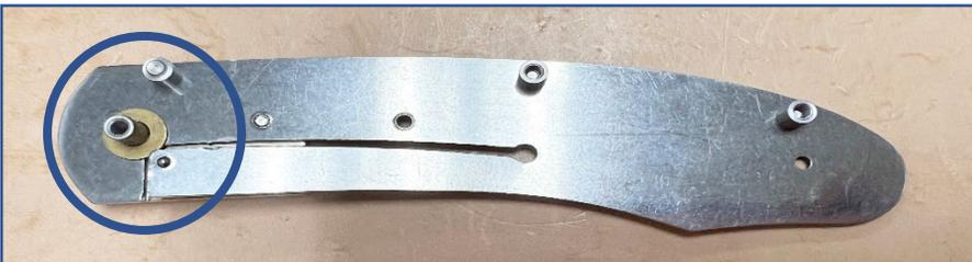
Place the bushing around the pivot pin and the remaining stop pin in place as shown in the photo.
