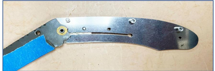
Place the blade over the pivot pin and bushing. Adjust the lock as needed to fit blade securely. Place remaining bushing onto pivot.
