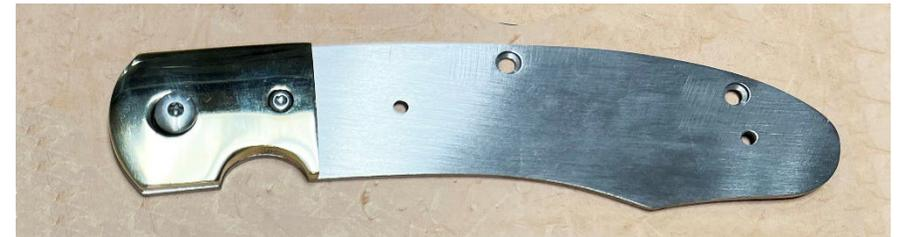
Attach bolster to right liner using remaining bolster screw and insert male pivot pin.
