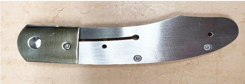
Attach one side of the bolster to the left locking liner by inserting the female pivot pin and screwing the bolster with the medium screw.
