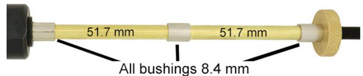
1. Assemble the bushings and barrels onto the mandrel referring to the image above.
