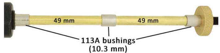
1. Assemble the bushings and barrels onto the mandrel referring to the image above.
