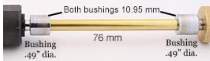
1. Assemble the blank and bushings on the mandrel as shown above. Since there is only one blank, you may need to use spacers in order to tighten the tube for turning.
