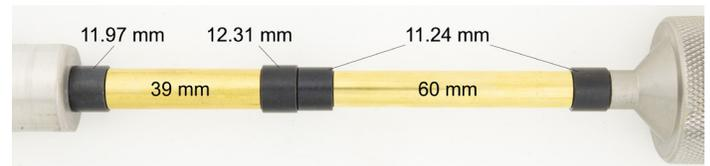
1. Assemble the bushings and barrels onto the mandrel, referring to the image above.
